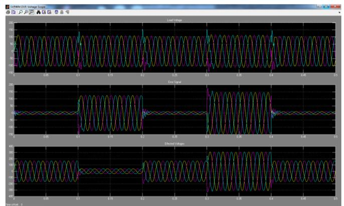
**Figure-8 Three phase voltage compensation.**
